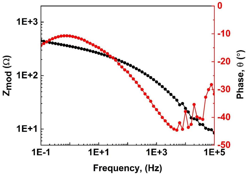
Figure6 : Bode plot of ECO MET 500LC sample after 7 days of immersion
