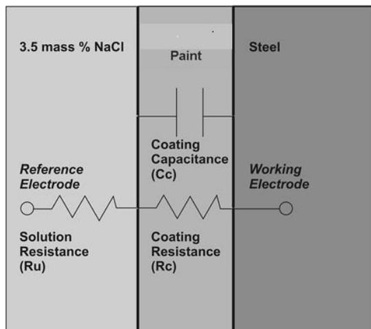
**Figure 10** :Equivalent circuit used for modeling
