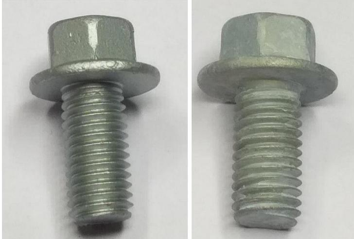
Figure 10 : Before and after salt spray test
