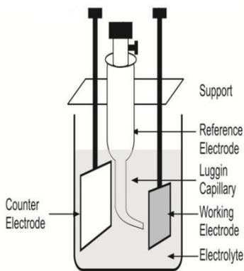
Figure 1: Electrochemical cell
