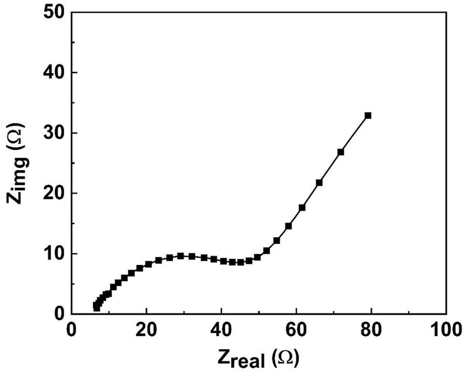
Figure5: Nyquist spectra of ECOMET 500LC sample just after immersion
