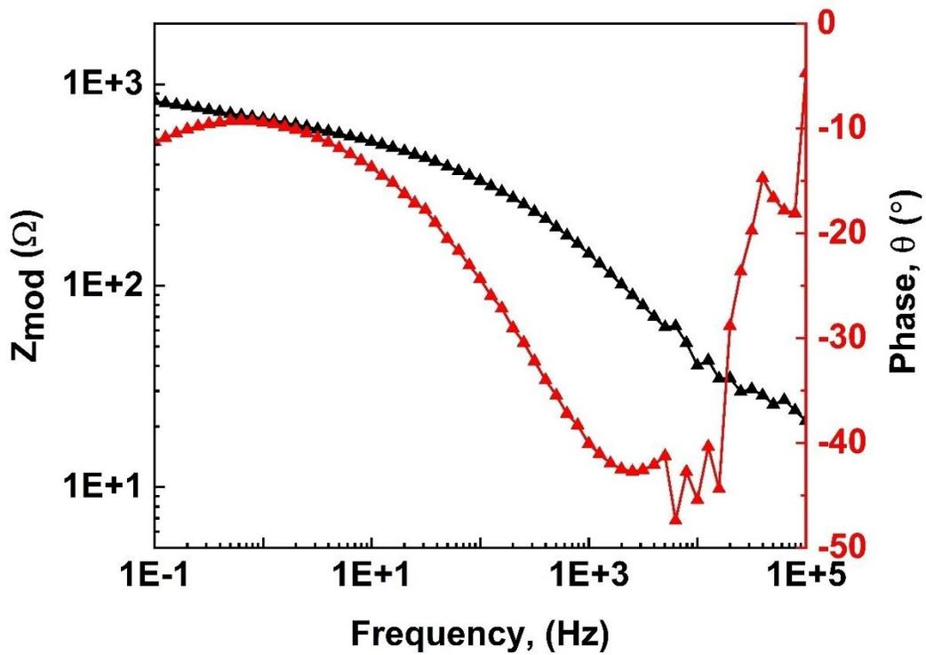
Figure8 : Bode plot of ECO MET500LC sample after 15 days of immersion.
