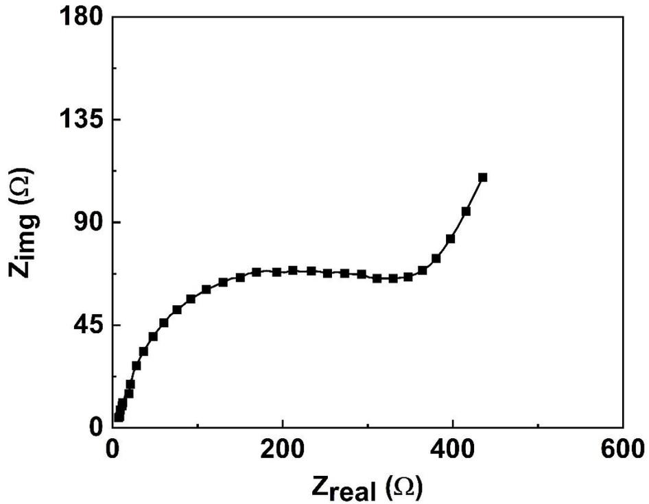
Figure7: Nyquist spectra of ECOMET 500LC sample after 7 days of immersion
