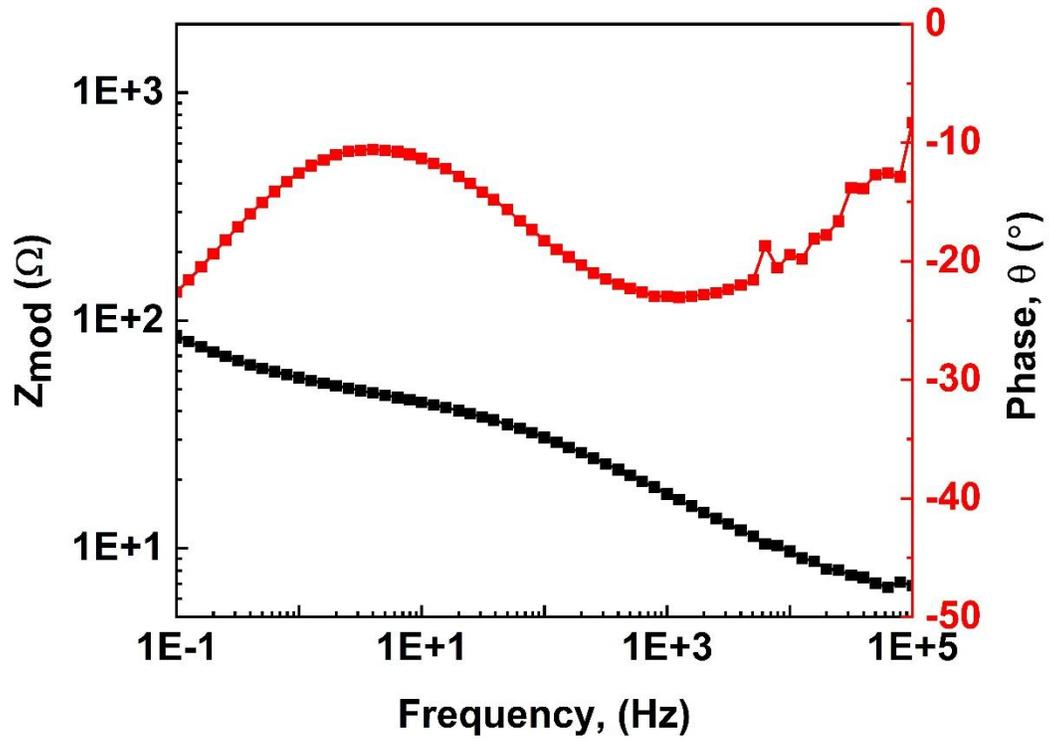
Figure4 : Bode plot of ECOMET 500 LC sample just after immersion
