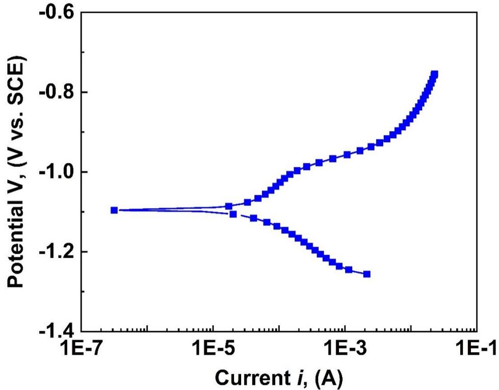
Figure 3: Potentiodynamic polarization of the Ecomet 500 LC in 3.5 % NaCl solution
